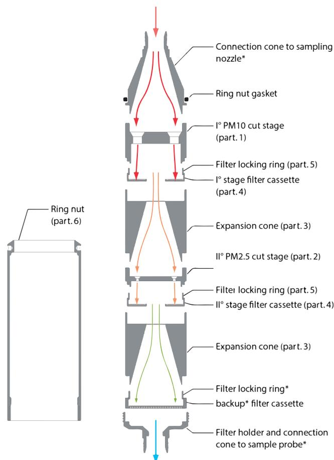
To meet the increasing requirements toward the fine particulate determination and progressive reduction of emission dust concentration, TCR Tecora added, to the already stated cyclone series realised according to USEPA design, the new multistage cascade impactor mod. MSSI.
