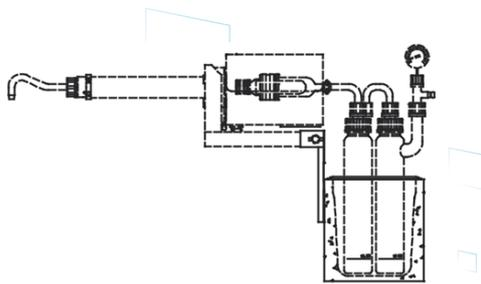
The cooling bath can be quickly connected to the heated through the support shown in the design.
